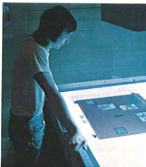
4. PHOTO NEGATIVES are aligned and checked on light table before printing plate is made.
